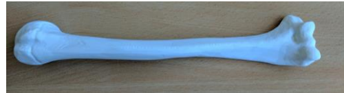
Fig. 4. 3D printed bone with RFID tag inside
